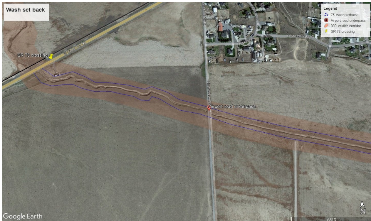
Figure 2. Map showing the wildlife overlay corridor through West Canyon, wash (highlighted in red) and the 75' wash setback in blue. Eagle Mountain City, Utah 2022 image.
