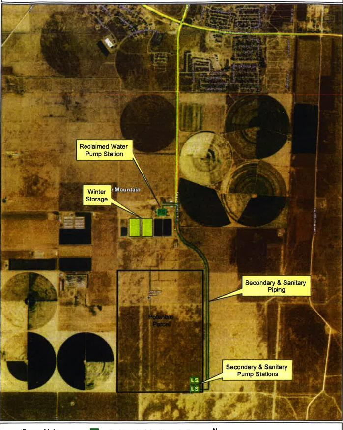
Sewer Main Reclaimed Water Pump Station N 0 1,000 2,000 4,000 Secondary System Sewer Lift Station
