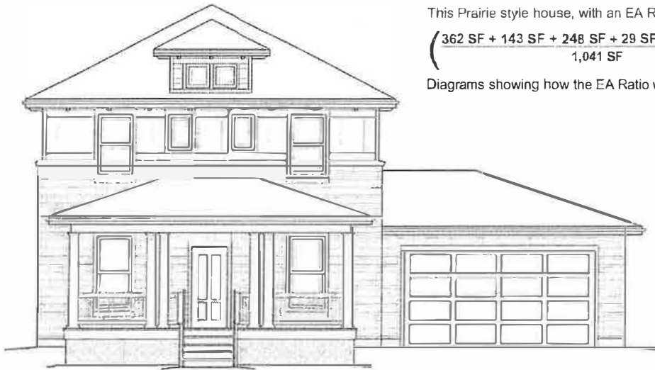
This image shows the siding elevation of the same house: it's EA Ratio is 0.57.
